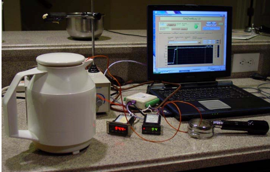
Picture 2. Thermos used for calibrating Themofilter
